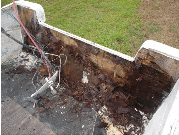
Figure 2 – Notice that the wood inside the transom was about the consistency of compost ready for the garden.
